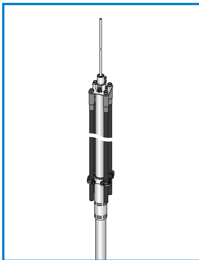
Figure 10 HVI®long Conductor installed outside the supporting tube - Complete
