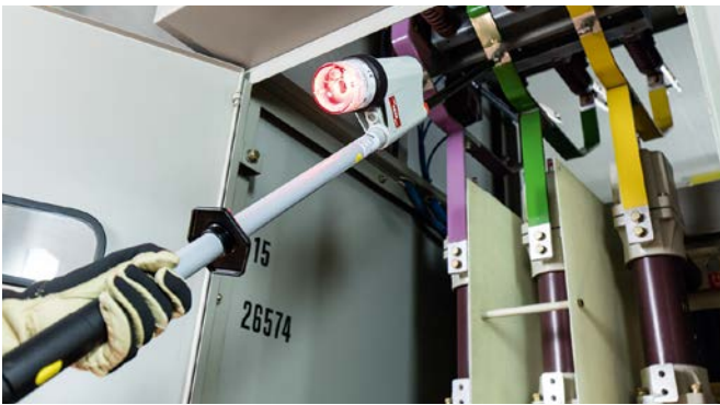
PHE4 voltage detector with visual and acoustic indication.
