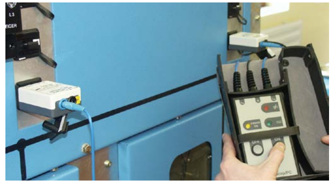
DEHNcap/PC-LRM phase comparator with two HR-LRM test adapters used in an HR switchgear installation
