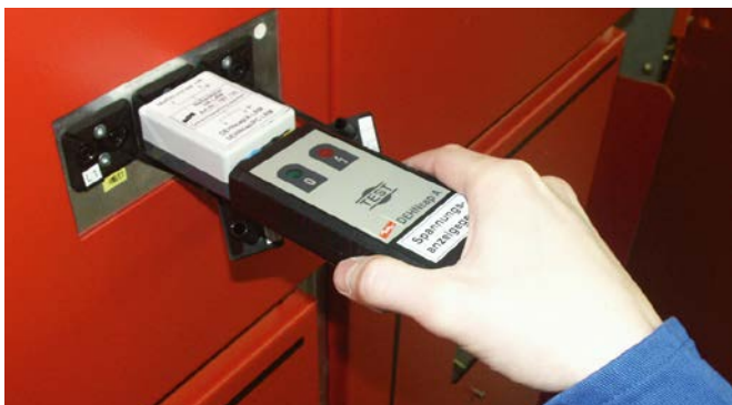
The HR-LRM test adapter for plugging an LRM indicator into a HR test socket.
