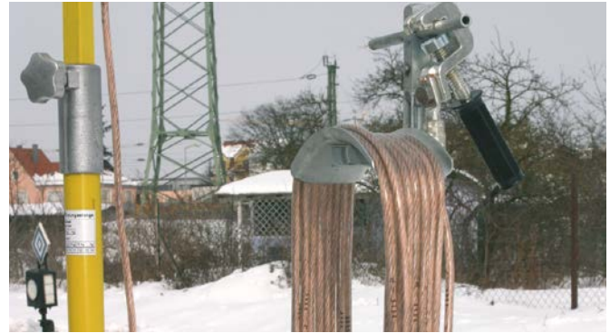
Earthing spike with coiled earthing cable.
