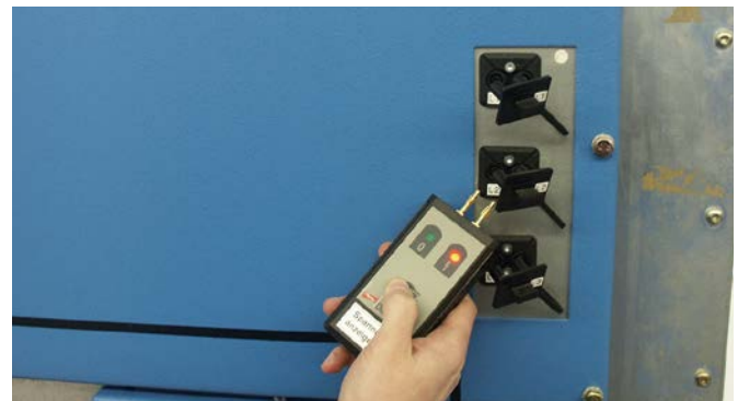
Self-test of a DEHNcap/A voltage indicator
